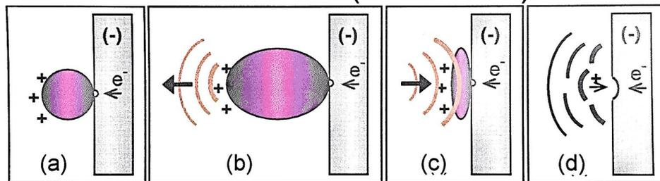
Physical process in PE. (a) Plasma formation around cathode, (b) plasma expansion and induction of shock wave, (c) collapse of plasma bubble due to electrolyte quench, and (d) explosive impact on electrode surface.
