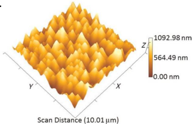
Textured surface and nanoparticles can only be created by anisotropic chemical etching:
