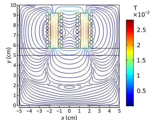
Magnetic field  $B$  of Ar MEIPS discharges with ferrite cores at 2 MHz (T)
