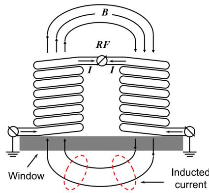
Schematic diagram of the magnetically enhanced inductive plasma source (MEIPS)
