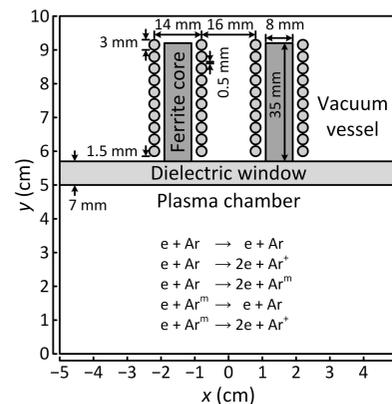
Schematic diagram of the simulation region of MEIPS
